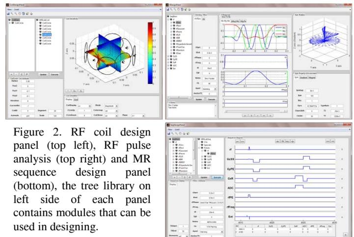
Figure 2. RF coil design panel (top left), RF pulse analysis (top right) and MR sequence design panel (bottom), the tree library on left side of each panel contains modules that can be used in designing.
